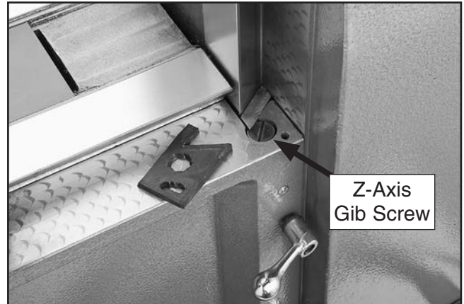
Figure 82. Location of Z-axis gib adjustment screw.
